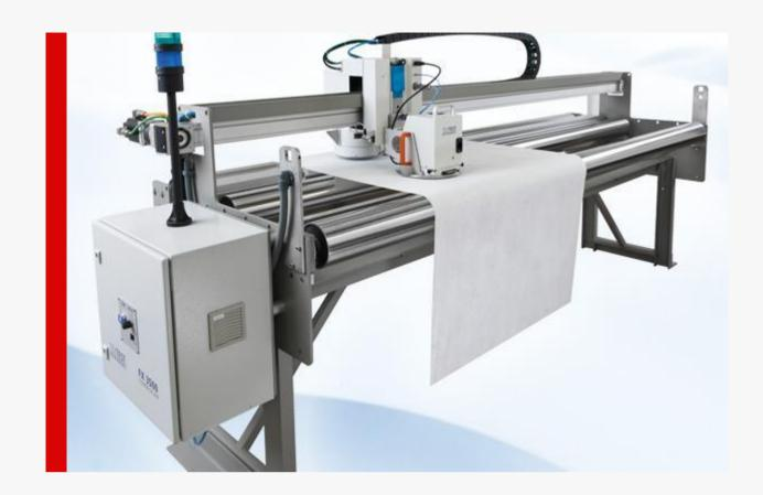
In order to achieve customer satisfaction and meet requirements, quality control and monitoring is provided through an on-line tester which continuously measures the air permeability and/or thickness as well as off-line on Palas Test rig, SEM and Porometer. Our processes are designed to provide the best in product quality, safety, and reliability.
