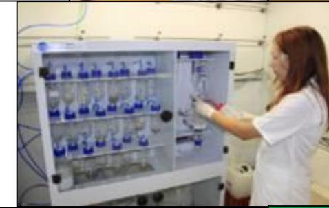
purification lab equipped with preparative HPLCs and lyophilization stations
