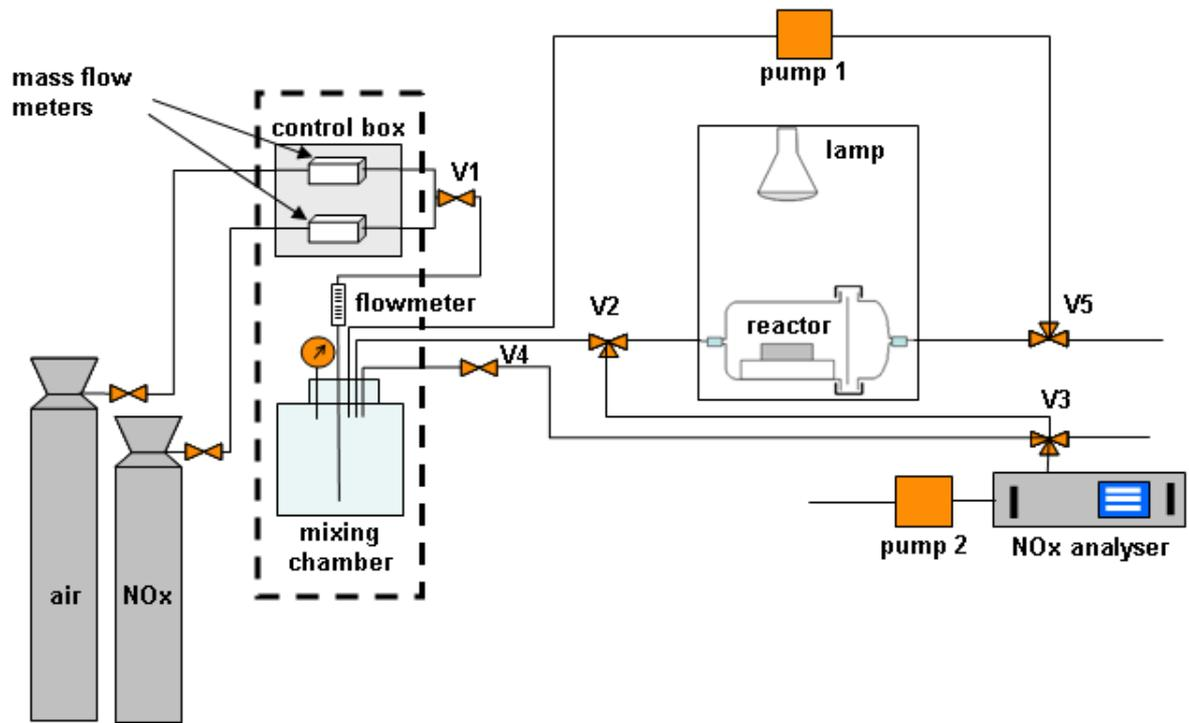
Figure 15- NOx gas recirculation test – A schematic view
