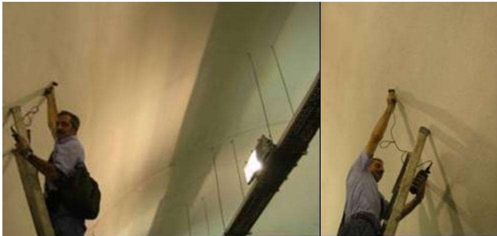
Figure 25 – Measurement of the light intensity, in the tunnel
