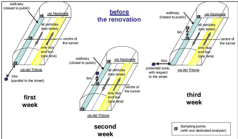
Figure 17 – Positions of NO<sub>x</sub> analysers, during the first campaign
