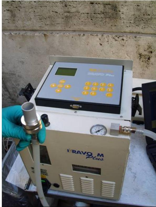
Figure 48 – TCR Tecora pollution check equipment, over the NOx analyser
