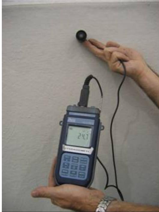
Figure 26 – Measurement in the tunnel, using the photo-radiometer
