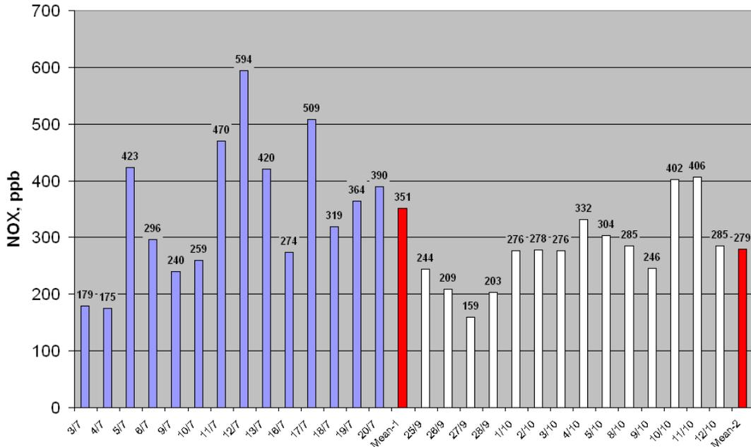
Figure 39 – NO<sub>x</sub> values in the centre of the tunnel, 1m
