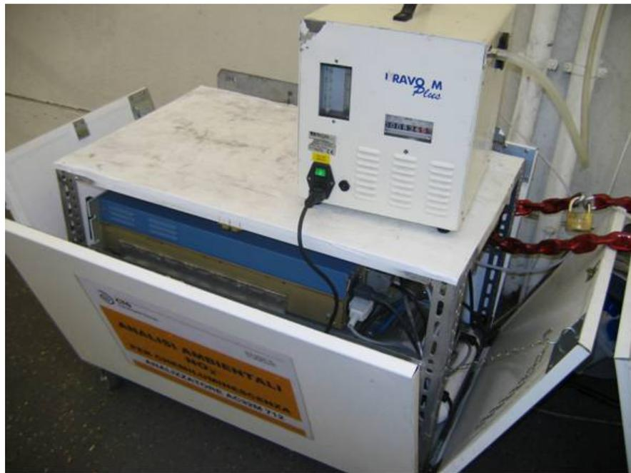
Figure 47 – TCR Tecora “Bravo M Plus” equipment, over the NOx analyser
