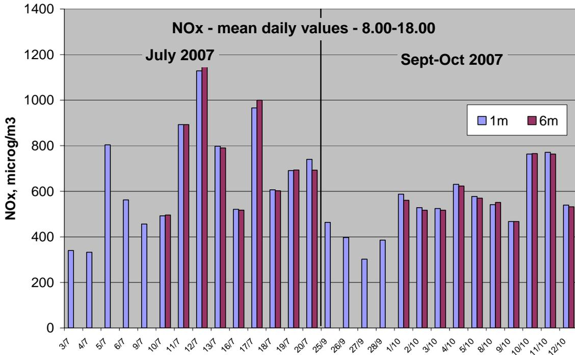
Figure 38 – Comparison of NO<sub>x</sub> values, in the centre of the tunnel (1 m and 6 m)
