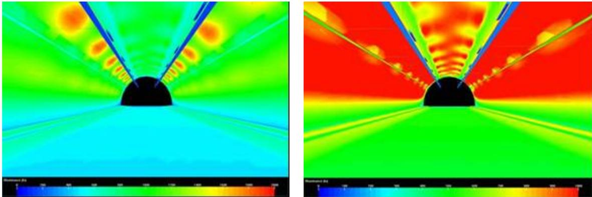
Figure 12 – Simulation design of lighting system: visible light irradiation (left) and UV-light irradiation (right)
