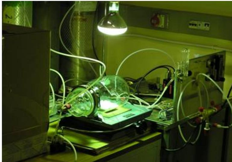
Figure 16 – NOx gas recirculation test – the light irradiation step
