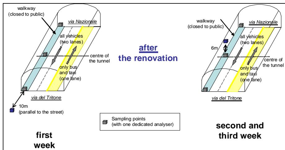
Figure 18 – Positions of NO<sub>x</sub> analysers, during the second campaign
