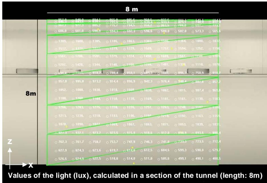
Figure 14 – Calculation of light irradiation, along the tunnel
