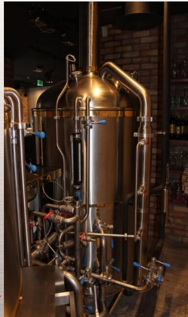
5,5 hl stainless steel brewhouse with brass design elements
