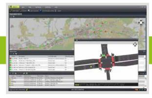
eDaptiva® is a multi-featured urban traffic management center. eDaptiva® provides monitoring, supervision, and adaptive control and meets different requirements of small, middle-sized or large urban areas. Basic system monitoring is available also via eDaptiva® web thin client in an online form of Invipo interface.
