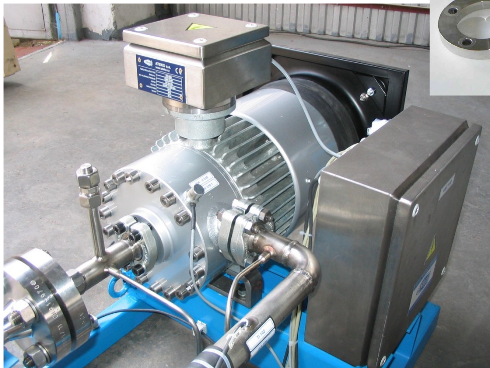
TC CEA – 9 kWe, 85 000 rpm (He, 75 000 rpm, Pin/out 80/95 bar, N= 11 kWe)
