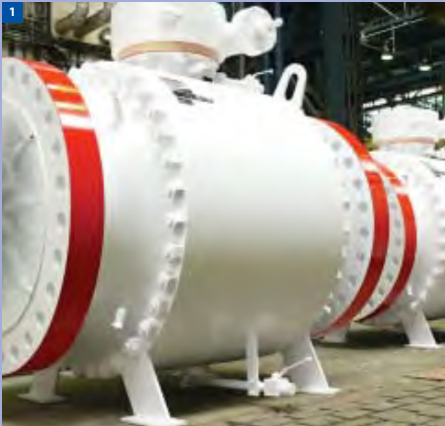
FOTO 1 – Ball valves nominal size 40", Class 600 designed for Turkish project, FOTO 2 – Ball valves nominal size 40", Class 600 with extension
